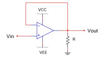
For the circuit in figure 1 with R = 5.1 K $\Omega$ , VCC = +12 V, VEE = -12 V, and the parameter values in section 6.1, answer the following questions:
