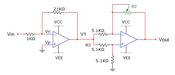
2. Analyze your circuit to prove that it has the gain as specified. If you find out that the magnitude of the gain somehow is not large as the gain magnitude for the circuit in Figure 2, explain why this is so.
