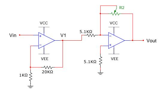
2. Analyze this new circuit to find the overall voltage gain Vout/Vin in one particular case when R2 = 8 K $\Omega$ .
